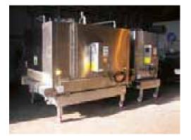
Air Cycle cooling-heating tunnels. Credit: FRPERC
